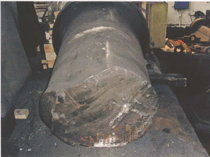
This piston rod broke because it was too cold and misaligned.
