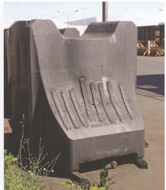
Broken upper counter-blow ram held together with straps for removal and eventual repair.
