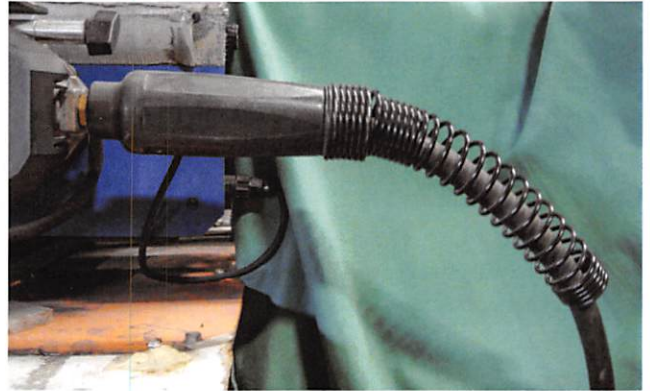
Spring liner wear can cause "birdnesting" of wire and clog the MIG gun.
