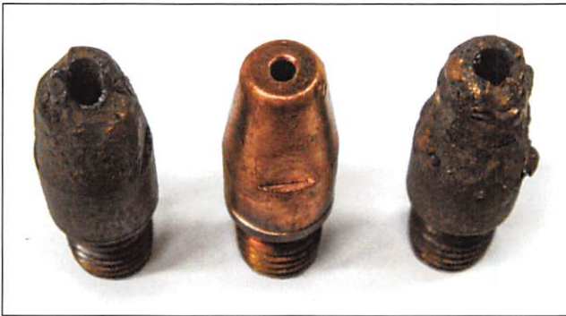
The MIG gun's tip gets the most wear of any part and should be replaced regularly.
