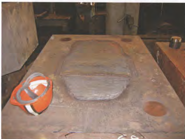
Example of finished, welded die
