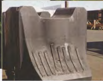
Fractured upper counter-blow rams (left and center) and drop hammer ram (right)
